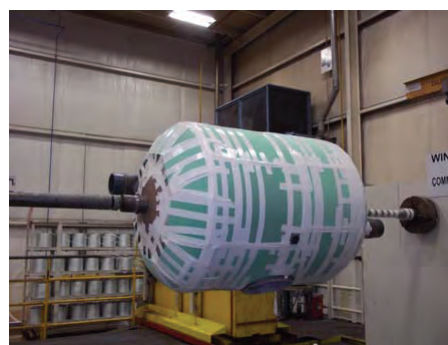
Insulated Vessel at Start of Winding
